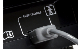
Fig.3 - Loopback connection to Duet.
