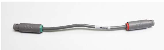
Fig.9 - Loopback cable for the USBLite system.
