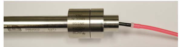
Fig.2 - Connection of ER3 to SPL Meter.
