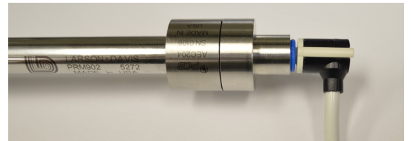
Fig.3 - Connection of 10D Probe to SPL Meter.
